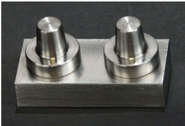
Fig. 1. The stainless-steel die containing 2 complete-crown, tapered abutment preparations abutments that provided the standardized master model to compare the defects associated with each of the elastomeric impression materials (base diameter of 12 mm; height from the shoulder margin of 8 mm; shoulder width of 3 mm; taper of 6 degrees; distance between the centers of the abutments of 20 mm).
