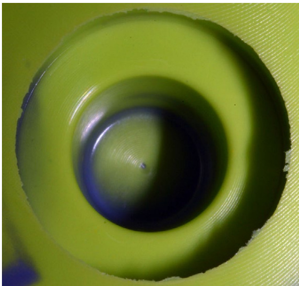
Fig. 3. Representative impression with an absence of bubble-like enclosed voids or open voids (polyether impression material).
